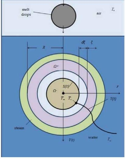
Fig. Scheme of calculated area of hardening of drops of a melt when driving in an air and aqueous medium:
