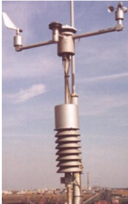
Fig. 3. Automatic meteorological station collecting and transmitting meteorological data
