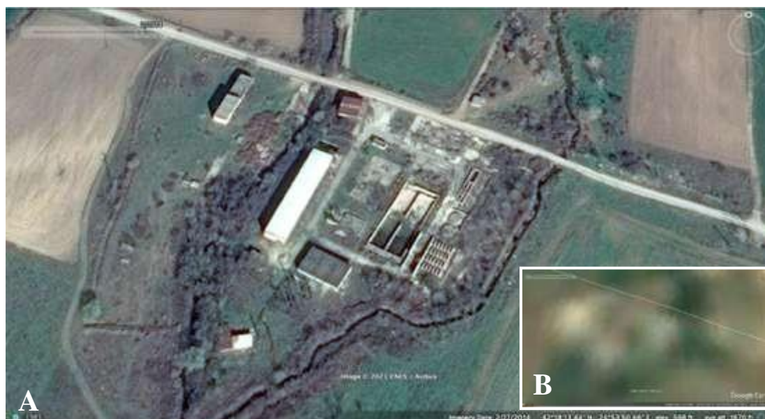
Fig. 6. (above) Site of former ISL uranium mining facility near Momino, (location B, Fig. 2). A) aerial view showing remaining mining infrastructure on 27 February 2014. The long building with the white roof housed air compressors; it is currently used as a cattle shed; B) inset - the same areal area shown in 6A during active mining. Image is “blurred”, i.e., censored, dated 31 December 1985. Images from Google Earth.
