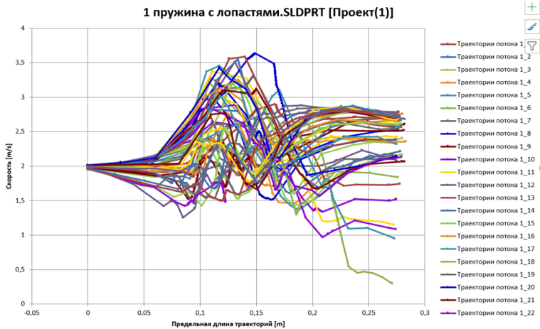
Figure 3. Graph of the dependence of the flow velocity on the length of the trajectory
