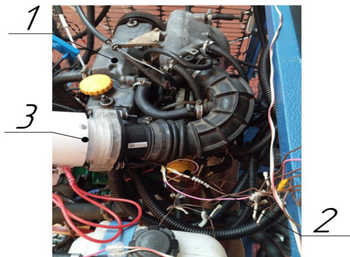
Figure 3. Internal combustion engine with magnetizing device and ozone generator:
