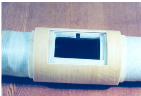
Figure 3. Glue-welded connection of biplastic pipes
