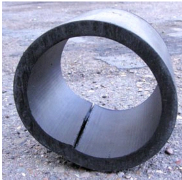
Figure 7. A sample of a spontaneously destroyed pipe
