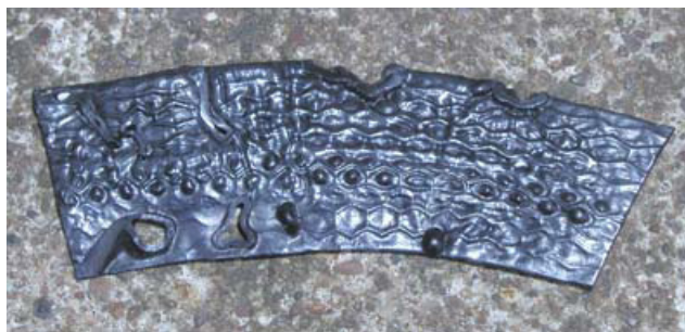
Figure 6. Pipe section after heating
