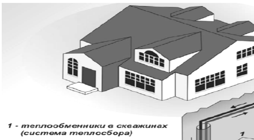
Figure 2. Schematic diagram of an autonomous heat supply system based on a closed-loop heat pump station with vertical ground heat exchangers
