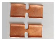
Figure 5. Blanks after deformation
