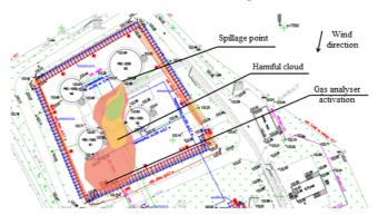
Figure 2. Scheme of the tank farm on the territory of Buzovyazovskoye oil field
