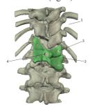
Figure 1. Customized navigation template top view at the creation stage. 1-patient's spine, 2-template body, 3-holes for fixation with Kirschner wires, 4-tube for osteotomy performance.
