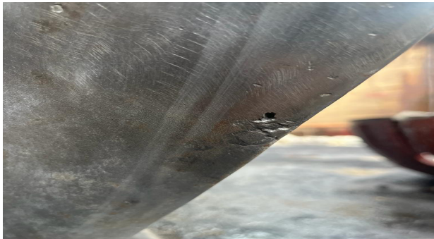
Figure 1. Wear of the blade edge of the nuclear container ship “Sevmorput”
