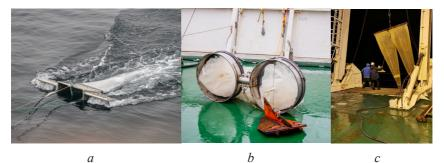
*Figure 1.* Equipment for collecting MP samples: on the sea surface - Manta neuston net (a), in the water column - Bongo 60 plankton nets (b) and DNS (c)
