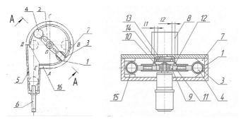
Figure 1. Impact test stand with braking section (AB)
