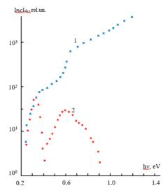
**Figure 2.** FP spectra(1) and Ic(2) for PbTe films obtained on a SiO2 –Si substrate. T=300K
