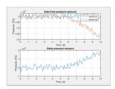
**Figure 9.** Variation of pressure in the pipelines and their differential at smooth leakage
