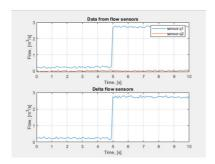
Figure 7. Flow rate variation in the pipeline during a sudden leak
