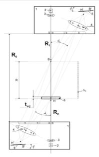
**Figure 1.** Structural scheme of the measuring bracket of the laser thickness gauge: 1 - laser distance gauges; 2 - semiconductor emitters; 3 - forming optics of the emitter; 4 - receiving lens; 5 - linear receiver; 6 - thickness standard; R1 -
