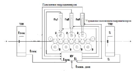
Figure 3. Gibon tensioning device (GTD) for metal strip drawing: TL1 and TL2 - laser thickness gauges, Hz1, Hz2, Hz3 - hydraulic cylinders, 2 - pressure rollers, 3 - support rollers, , – strip thickness, before GNU, after GNU. KY- control unit, minimum permissible drawing thickness entered by the operator
