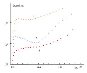
Figure 4. FP spectra for PbS films obtained on polycor; 1 - after heat treatment for 10 min in an oxygen-containing atmosphere; 2 - after heat treatment for 20 min; 3 – after heat treatment for 20 min and plasma etching.
