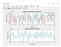
**Figure 4.** Values of pressures in the pipelines and their difference in the absence of leakage
