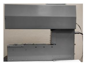
Figure 2. Laser thickness gauge TL-3. Dimensions W x H x L, 185 x 596 x 760, mm, weight 75 kg.
