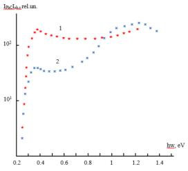
**Figure 1.** Spectra of phase transition (1) and Ics (2) for PbTe films obtained on glass-ceramic substrate. T=300K
