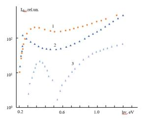
Figure 3. Photo-EMF spectra for PbS films obtained on polycor. 1 - after heat treatment for 10 min in an oxygen-containing atmosphere, 2 - after heat treatment for 20 min and plasma etching, 3 - after heat treatment for 20 min.
