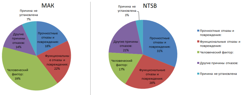
Diagram 2. Distribution by main groups of failures and damages according to IAC (left diagram) and NTSB (right diagram).
