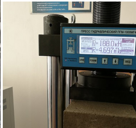
Figure 5. Compression test of hollow wall stone
