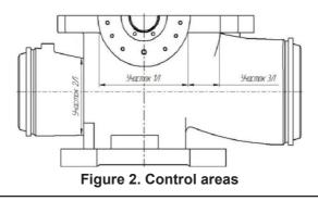
The control is carried out for the presence of various defects in the casting of the body, the most common is a defect of the "looseness" type - a casting defect in the form of an accumulation of small shrinkage cavities [5]. A sign of this defect is that the image of the defect consists of a chain of small images.
