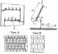
a) sieve tray with prosechno- exhaust openings and baffle elements
