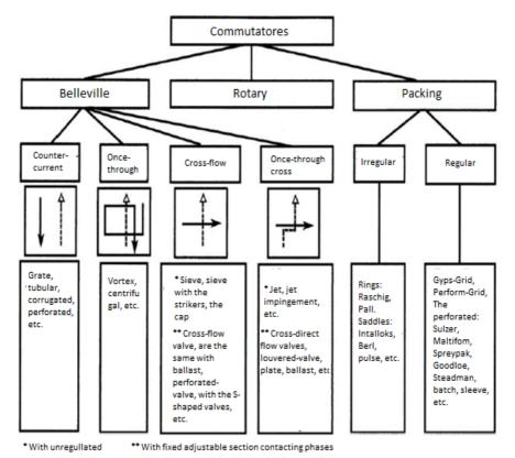
Figure 1 Classification of contact devices
