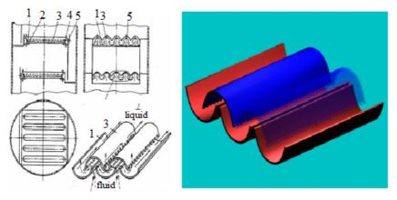
1 – gutter; 2 – supporting rails; 3 – caps; 4 – pins; 5 – drainage Figure 2 Plate with grooved (tunnel) caps
