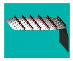
b) sieve tray with perforated elements (punched perforation) with perforated vertical partitions
