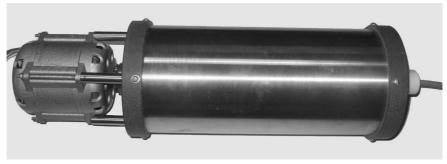
Fig. 3. The reactor part of the ozone generator
