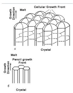
Figure 5 - Cellular structure (a) and pencil (columnar) structure (b) [10]
