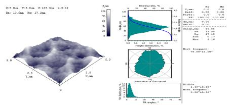
Figure 2 - 3D image of AlFeCrMnSiCu coating
