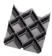
Figure 7 - Cellular dislocation structure in axonometric projection [22]
