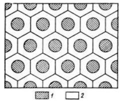
1 - upward movement, 2 - downward movement Figure 6 - Layout of Benard cells [19]
