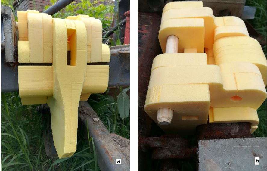
Figure 7 – A prototype of a quick-detachable chisel attachment made of foam and mounted on a subsoiler frame (rack not shown). Shown: a – adapter of the working body 6 and 7 the first part of the split unit; b – 7 the first part of the split unit and the adapter of the implement 6.
