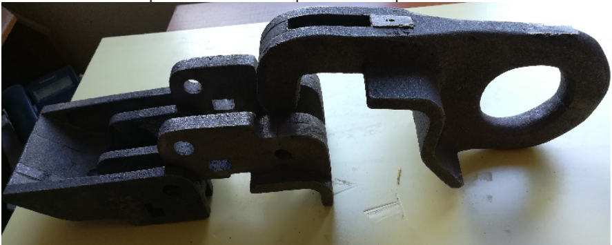
Figure 8 – The parts of the adapter of the working body 6 made of metal (the ring is cast for another purpose) of the first part of the detachable unit 7, interconnected by the axis 16.
