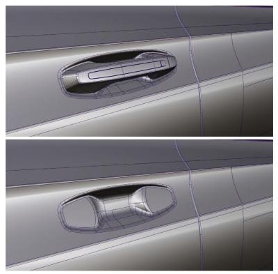
Fig. 2 Door handle and the place of its attachment to the surface of the door panel (Alias 3D model)
