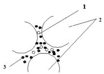
1 – gas pore; 2 – air entrained pore; 3 – capillary pore; Figure 1 – Physical model of the porous structure of composite aerated concrete
