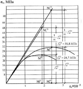
Fig. 3. Experimental curves  $\sigma_c - \varepsilon_c$  taking into account the degree m = 1.
