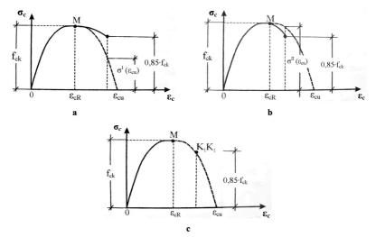
**Fig. 4. Diagrams**  $\sigma_c - \varepsilon_c$  for different values of the modulus  $E_2$ :  $\mathbf{a} - E_2 > 0$ ;  $0.85 \cdot f_{ck} > \sigma'(\varepsilon_{a})$ ;  $\mathbf{b} - E_2 < 0$ ;  $0.85 \cdot f_{ck} < \sigma''(\varepsilon_{a})$ ;  $\mathbf{c} - E_2 = 0$ .
