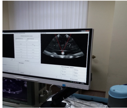
Ultrasonic picture of the thermal ablation zone (round shape) of the phantom (PAG-3) at a radiation intensity of 8.2 kW / cm 2 averaged focus up to 0.6 mm and an exposure of 1000 ms.
