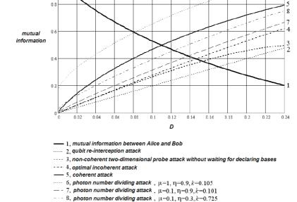
Fig.3. Mutual information I (D) AB (curve 1) and I (D) AE for different BB84 protocol attack strategies (curves 2–8)
