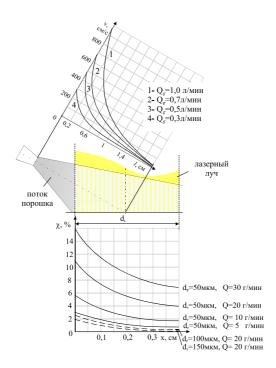
Fig 1. The fraction  $\chi$  of the radiation power that is absorbed by the powder stream and the velocity distribution v of the powder along the x axis of the stream for different particle diameters d, at various transport gas consumptions  $Q_g$  and powder Q.
