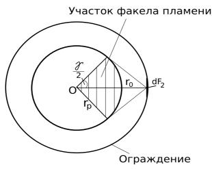
Fig. 3 The surface of the flame plume participating in heat exchange with the elementary site dF, (top view)
