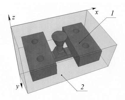
**Figure 1.** The structure of the modeling area: 1 is mold cavity filled with metal (region M); 2 is casting shape (region F).
