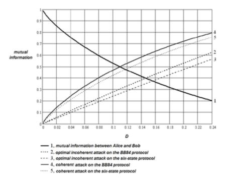
Fig.4. Mutual information I (D) AB (curve 1) and I (D) AE for various strategies of attacks on a protocol with 6 states (curves 2–5)
