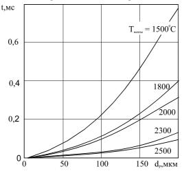
*Fig. 3.* The melting time of VK3 powder particles depending on their diameter at different temperatures of the melt bath.
