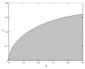
**Fig.2.** The field of parameters  $\eta$  and  $\mu$ , where the attack will be successful when replacing the original channel with losses to an ideal
