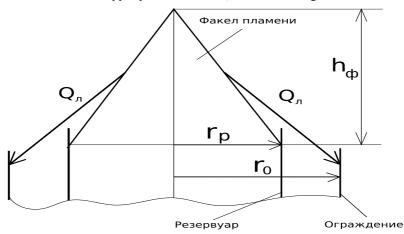
**Fig. 1.** Fire model in a tank with a protective wall:  $r_0$  – radius of the heated surface of the cylindrical wall of the fence, m;  $r_p$  – the radius of the cylindrical tank, m;  $Q_s$  – heat flux transmitted by radiation from the flame to the surface of the upper part of the fence, W;  $h_\phi$  – flame height, m.
