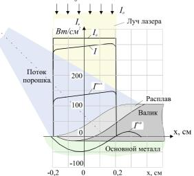
Fig. 2. Distribution pattern of laser radiation intensity and heat  $(P = 4kW, dL = 4mm, Q = 10 \text{ g} / \text{min}, Qg = 1 \text{ l} / \text{min}, dP = 50 \text{ mkm}, Zc = 1.5 \text{ cm}, dc = 15 \text{ mm} \text{ and } \alpha = 45^{\circ}).$
