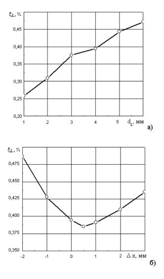
Fig. 4. The dependence of the mixing coefficient  $\xi_L$  on the beam diameter (a), the displacement of the laser beam relative to the center of powder supply (b) at  $P_L = 3 \text{ kW}, \text{ v} = 1 \text{ cm/s}, Q = 20 \text{ g/min}$
