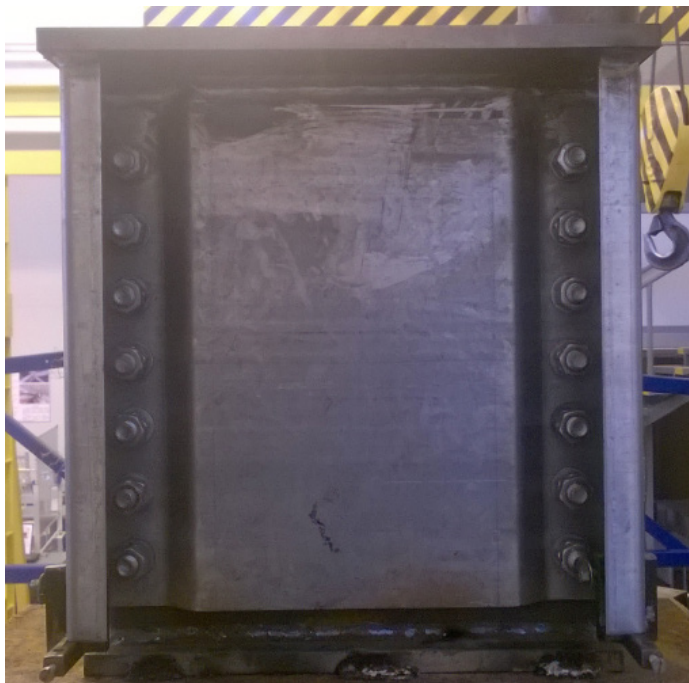
Fig. 1. The prototype of the bolt connection node
