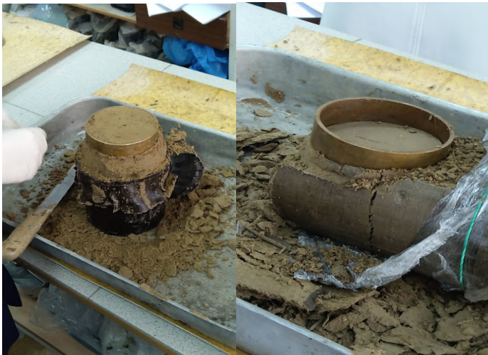
Figure 2. Sampling in the vertical and horizontal directions
