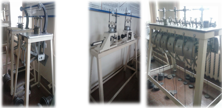
Figure 3. Compression device (odometer) and system seal “Hydroproject”
