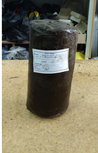
Figure 1. Sample of undisturbed soil with natural moisture
