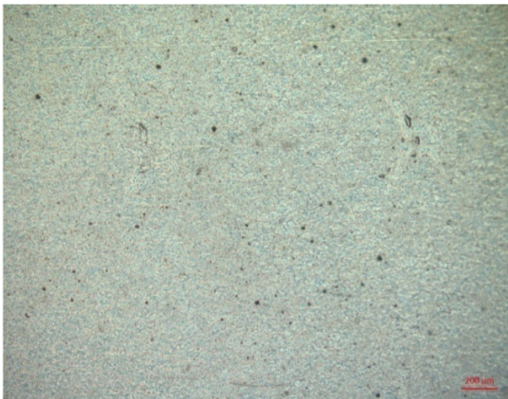
Fig 4. 2% shungite film after exposure to 200 nm radiation
