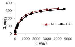
Fig. 2. Adsorption isotherms of phenol on ACF and GAC
