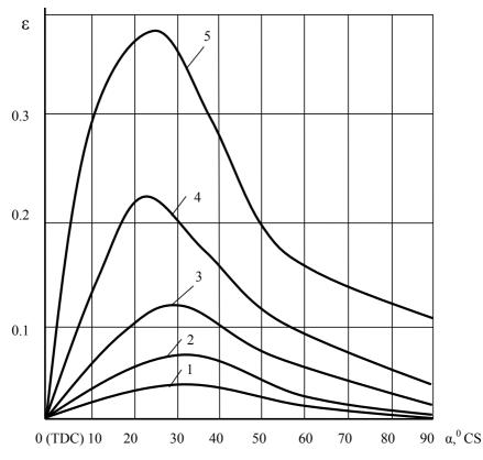
*Fig. 3.* Variation of integral degree of flame blackness by experience of marine diesel 6  $\Psi$  44/36 by power data: 1 – idling; 2 – 25% of Nenom; 3 – 50%; 4 – 75%; 5 – 100%
