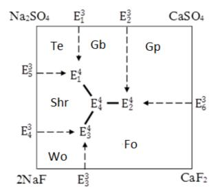
**Fig. 2.** Schematic diagram of phase equilibria of the Na,  $Ca//SO_{4^{\circ}}F - H_2O$  system at 50°C, constructed by the translation method
