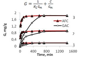
*Fig. 1. Kinetic curves of phenol sorption on ACF and GAC. Phenol concentration, mg/l: 0.6 (1), 2.4 (2),4.6 (3)*
