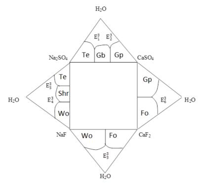
**Fig. 1.** Diagram of phase equilibria of the Na, Ca// SO<sub>\*</sub>  $F - H_2O$  system at 50°C at the level of a three-component composition in the form of a "Scheme" of a prism
