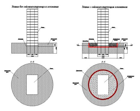
*Figure 8 -* Design scheme of building models with traditional seismic reinforcement and with a seismic insulating base
