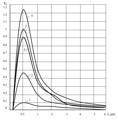
Fig. 2. Variation of spectral optical thickness of flame in marine diesel 6 ChN 24/36 by power 100% from Nenom: 1 - TDC; 2 - 200 CS after TDC; 3 - 400; 4 - 600; 5 - 800
