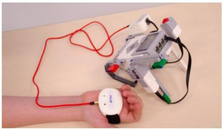
Fig. 1. Electromyogram Sensor in BiTronics Lab
