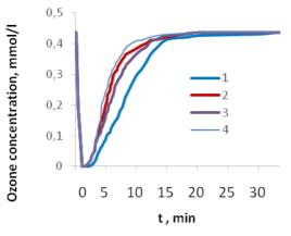
Fig. 3. Kinetic curves of ozone concentration at the outlet of the reactor in ozonation of phenol solution (1), phenol solution in the presence of ACF (2) and GAC (3), obtained after adsorption. Ozone concentration in the blank run with distilled water (4). Cphenol 200 mg/l.
