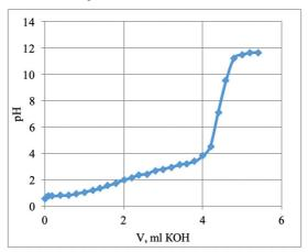
Fig. 1. The integral titration curve in water of a mixture of  $HA_1$  and  $HA_2$  acids with an aqueous solution of potassium hydroxide (the abscissa axis is - V ml KOH, OH, the ordinate axis is the pH of the solution)
