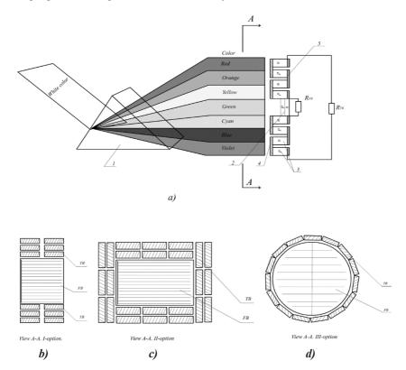
Figure 2 [16]. Optical layout of a selective photo thermal converter a) 1-prism, 2-photoelectric converter (PC), 2-p- and n-branches of the thermal converter (TEC), 3-hot switching plates of the TEC, 4-cold switching plates of the TEC, b, c, d): - respectively, three options for the location of the photovoltaic battery (PC) and thermopile (TP) along section AA: I, II, III variant.
