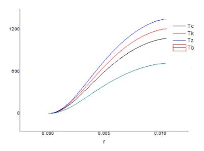
Figure 3. Temperature curves: Tb - barium, Tk - potassium, Tz - cesium, Tc -maximum temperature of graphite crystal in the center of the substrate to periphery
