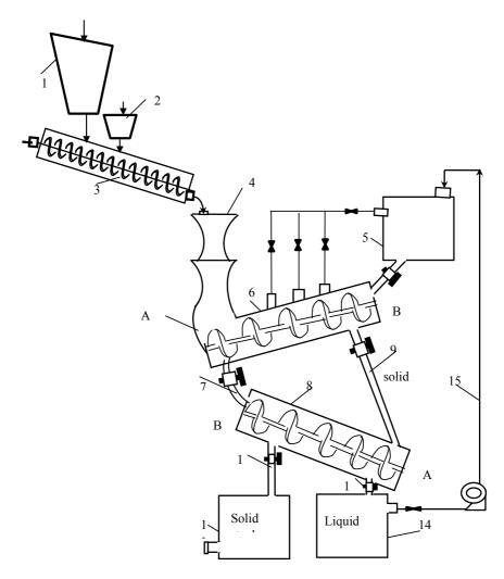
The equipment included in two knegs: 1 – bunker for cotton and cocoon; 2 – bunker for Siyazan clay; 3 – sneg (1); 4 – dozator for mixture (storage) of cotton and Siyazan clay; 5 – geothermal or mining DEP reservoir; 6 – sneg (1); 7 – sneg (2) to sneg (3); 8 - sneg (3); 9 - sneg (2 solid mixture from) to snek (3); solid mixture from 11 – snek (3); solution from 12 - snek(3) to common liquid line; 13 - solid mixture to use; 14 - liquid to use; 15 – liquid product to reuse.
