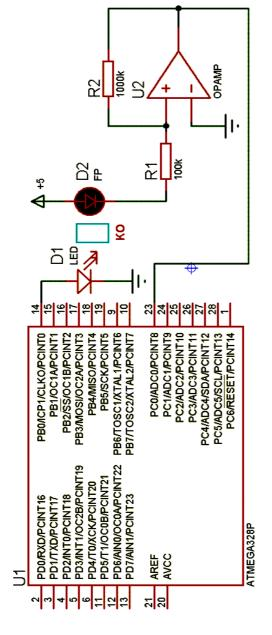
Fig. 2. Relative humidity sensor
