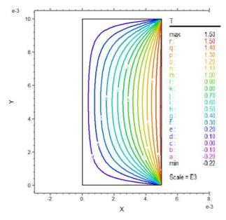
Figure 2. General graph of temperature field distribution in reaction cell
