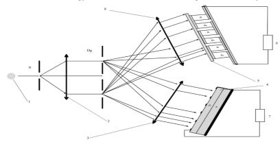
Fig. 1 [14]. The distribution scheme of light radiation on the surface of photovoltaic and thermoelectric converters
