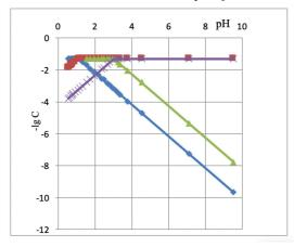
**Fig. 2.** Logarithmic pH-diagram of a mixture of 0.05 M HA<sub>1</sub> and 0.05 M HA<sub>2</sub>.  $K(HA_1) = 10^{-1}$  mol/L;  $K(HA_2) = 10^{-3}$  mol/ (abscissa axis –pH values; ordinate axis – logarithm of the concentrations of all equilibrium particles). Row  $1 - \lg[HA_1]$ ; Row  $2 - \lg C(A_1)$ ; Row  $3 - \lg C(HA_2)$ ; Row  $4 - \lg C(A_2)$ .
