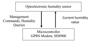
Fig. 1. Structural and functional diagram of a transmitting device for continuous monitoring.
