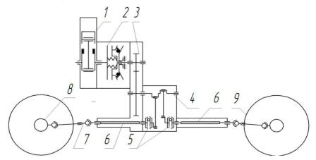
Fig.1 The kinematics of an elementary impulse type transmission for all-wheel drive (ATV)
