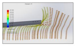
Fig.5 - Wrapping a wing model without a tip (angle of attack 4 degrees)
