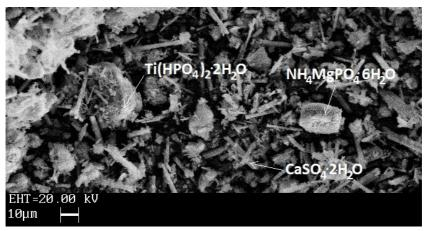
Fig.2. SEM image of composite titanium phosphate obtained by precipitation of 10% H3PO4
