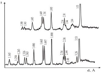
*Fig.1.* Radiographs of compositions obtained from oxides with the original ratio TiO2:SiO2: 1-1:1; 2 – 1:0.1.
