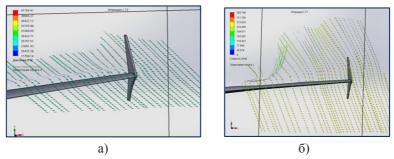
*Fig.* 7 - *Wrap around the wing model with the tip of the "Witcomb wings"* (*a - angle of attack 4 degrees; b - angle of attack 17 degrees*)
