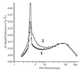
*Fig.3. BJH* pore distribution curve for composite phosphate, obtained by treatment with phosphoric acid concentrations of 1-20%, 2-10%.
