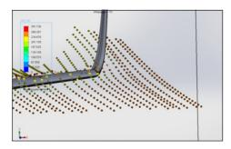
*Fig.6 - Wrap around a wing model with a blended winglet tip (angle of attack 4 degrees)*
