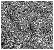
**Figure 2** - The microstructure of the cemented layer of steel 20X2H4A after heat treatment  $\times$  5000, the distance from the surface is 0.06 mm
