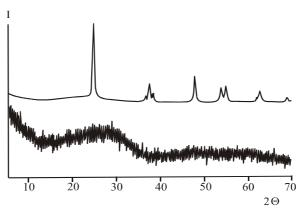
*Fig. 3.* Diffractograms of the composition obtained from titanium hydroxide and silicon oxide (lower), as well as calcined composition at 850 °C (upper).
