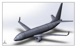
Fig.2 - 3D model of the Boeing-737-800 with blended winglet tips
