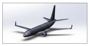
Fig.3 - 3D-model of the Boeing-737-800 with Split-tip tips
