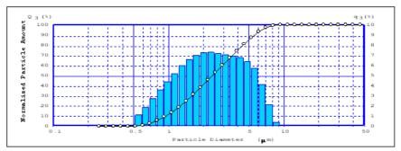
Fig. 5. Particle distribution after mechanical activation of a mixture of titanium hydroxide and silica.
