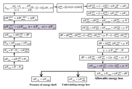
Figure 1. Block diagram of an improved algorithm for calculating the standard value of losses EP based on the combined approach, taking into account losses from leakage currents
