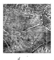
Distance from the surface, mm: a - 0.04; b - 0.12; c - 0,27; d - 1.50 Figure 1 - The microstructure of the cemented layer × 5000, steel 20X2H4A 国际会议
