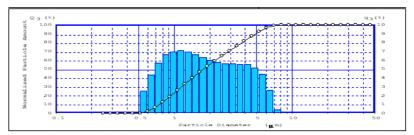
*Fig. 2.* Particle distribution after mechanical activation of a mixture of titanium oxide and silica.
