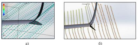
*Fig.9 - Wrap around a wing model with a "double feather" tip (a - angle of attack 4 degrees; b - angle of attack 17 degrees)*
