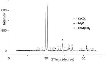
Fig. 1. Phase composition of thermally activated dolomite according to X-ray diffraction data
