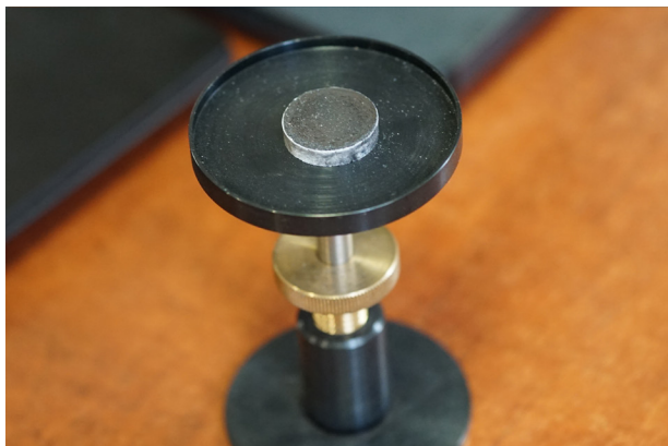
Figure.2. Coal sample prepared in accordance with GOST
