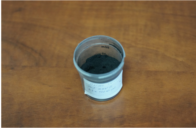
Picture. 3. Ground coal dispersion 315 microns prepared for testing
