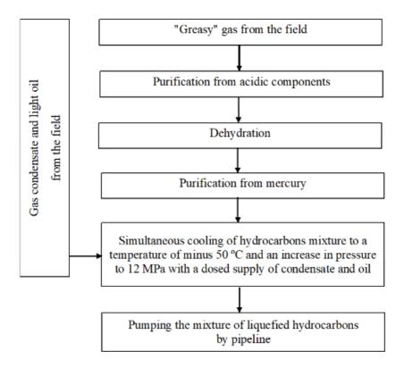
*Figure 1 - Scheme of the technology for producing a mixture of liquefied hydrocarbons [3]*
