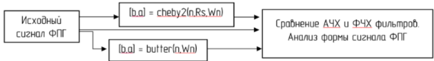
Figure 5 - Schematic representation of the process of filtering the signal with Butterworth and Chebyshev filters.
