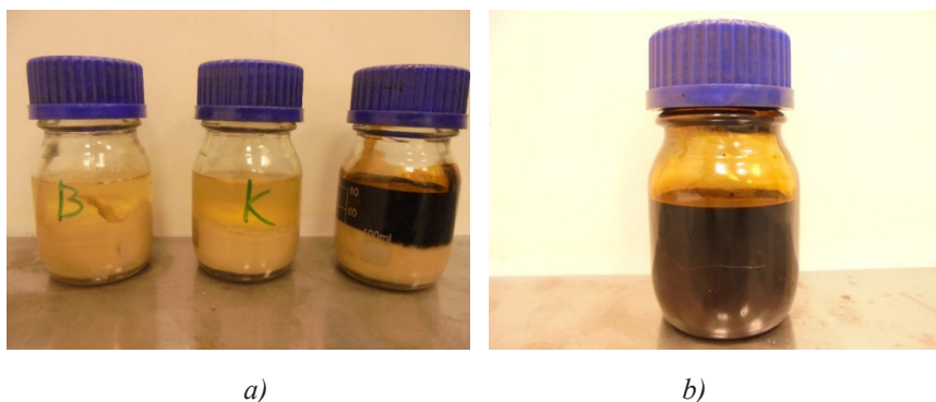
Figure 5 - The state of NOE contact on the emulsifier E1 8-9% with formation water (B), hydrochloric acid (24%) (K) and oil (H) for a period of time from 1 h to 24 h (a); dilution of NOE with oil (b)
