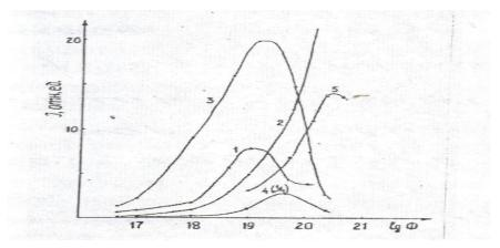
Fig. 2. Dependence of the intensities of the PL bands 550 (1), 660 (2). 840 (4) and GL 660 (3), 460 nm (5) from neutron fluence
