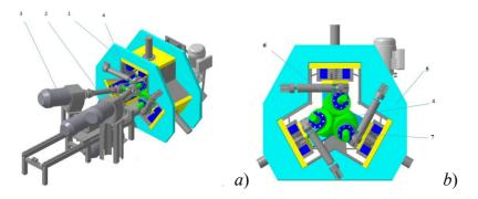
1 - work stand, 2 - spindle 3 - electric motor, 4 - work rolls; 5 - bed frame, 6 - pad, 7 - wedge
