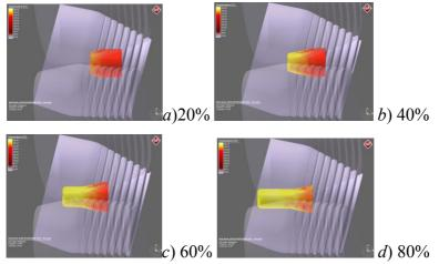
*Figure 2 - Picture of the distribution of the temperature field in the workpiece when pressing rods of aluminum alloy D16 on RSM with helical rolls*
