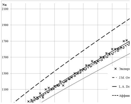
*Figure 1 -* Dependence of the dimensionless heat transfer coefficient of a turbulent rotational flow according to the law of a solid body at Pr = 0.7
