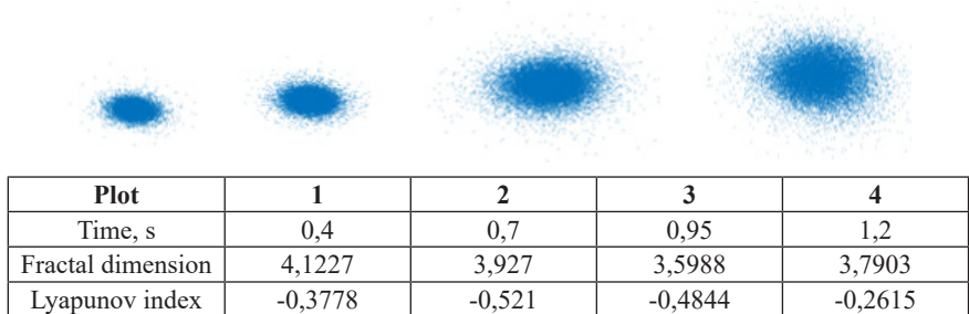
Figure 9. Attractor formation during tool plunge into the workpiece. Steel 45, cutter VK8, V = 15 m/min, a = 0.2 mm, c = 2 mm. Free cutting.
