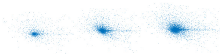
Figure 5. Time phase portrait of the VAE signal at friction along the Z-axis
