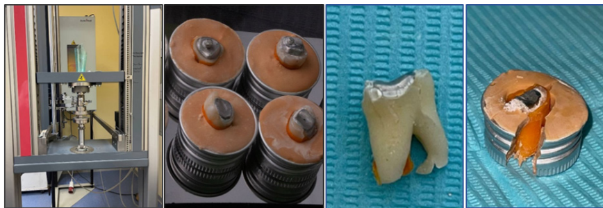
Figure 2. A model for testing the strength properties of teeth on a machine Zwick Roell Z 010
