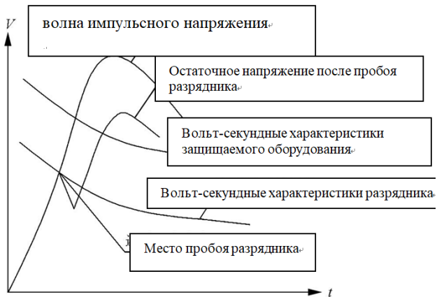
Figure 2. Coordination of insulation based on arrester protection
