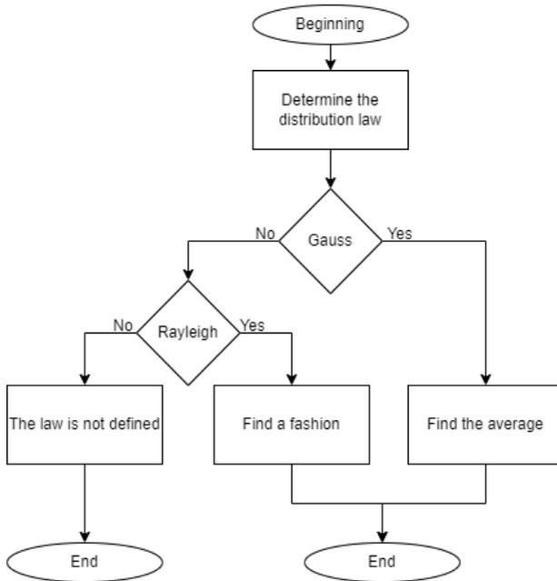
**Figure 3.** Algorithm for improving the quality of processing measurement results
