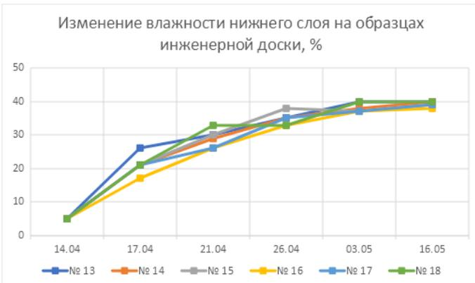
**Figure 5.** Change in the moisture content of the lower layer on samples of engineering boards, %
