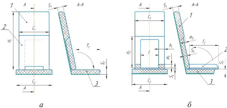
**Figure 4.** Method 2 of chair adaptation in the initial state (a) and after transformation (b).
