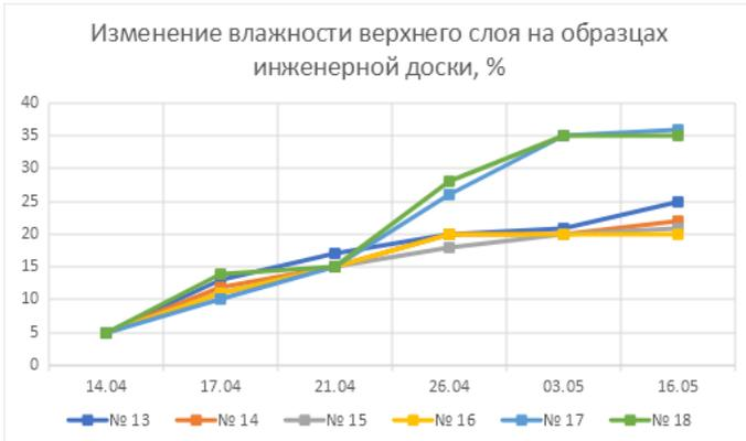
**Figure 4.** Change in the moisture content of the top layer on samples of engineering boards, %
