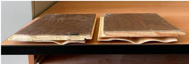
**Figure 7.** Detachment of the bottom layer of samples of parquet boards No. 7 and No. 8
