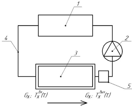
**Figure 2.** Functional model of pre-start engine heating at the heat accumulator discharge: 1 – engine; 2 – pump; 3 – heat accumulator; 4 – connecting hoses; 5 – electronic control.
