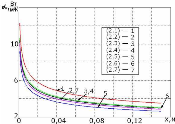
**Figure 1.** Distribution of the convective heat transfer coefficient along the height of the plate. The numbers indicate the curves corresponding to formulas (1-7), respectively. Curves 3 and 4, 2 and 7 overlap in the figure.
