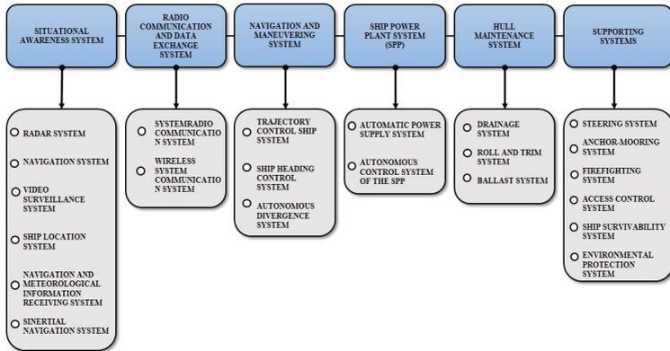
Figure 1. List of ship subsystems according to RMRS
