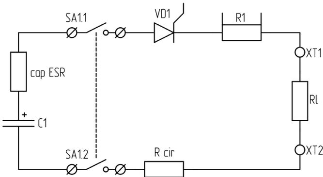
**Figure 1.** Schematic diagram of an electroexplosive installation, taking into account parasitic elements in the form of lumped parameters.
