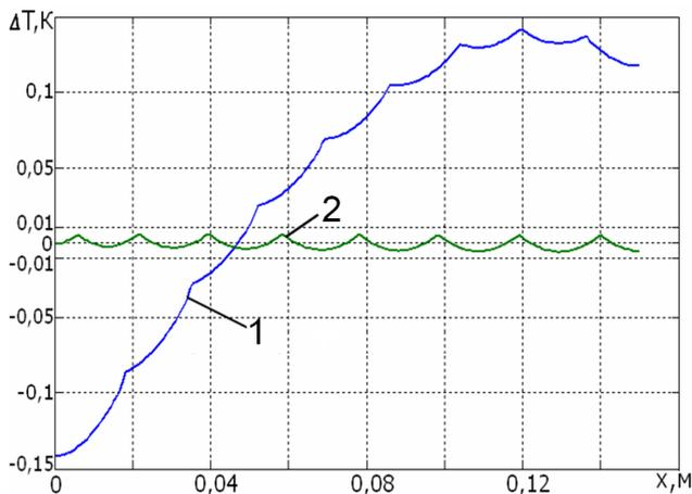
**Figure 4.** Temperature distribution over the surface of a vertical copper plate 1 mm thick: 1 – uneven heater; 2 - uniform heater.
