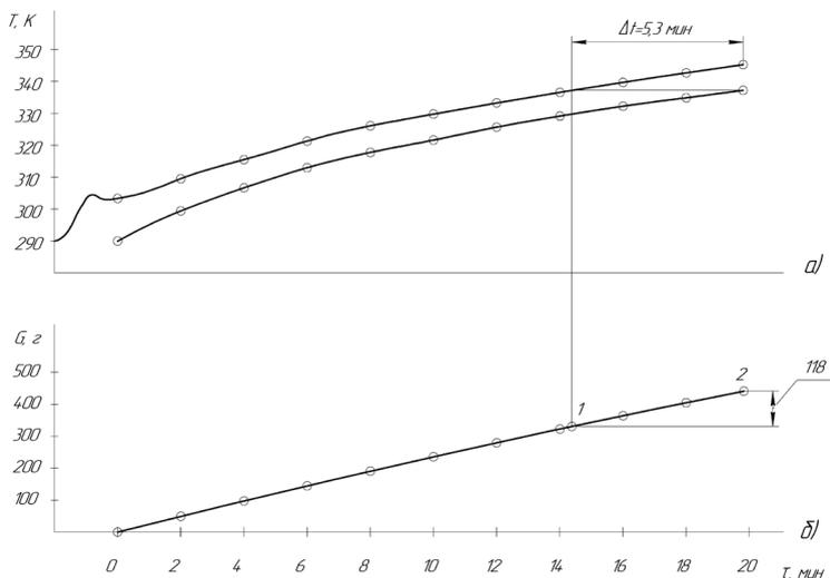
**Figure 5.** Engine temperature dependence on: a) fuel consumption b) engine pre-start heating period: Point 1 –the cooling liquid heating time to the operating temperature with pre-start heating. Point 2 – heating period without pre-start heating.
