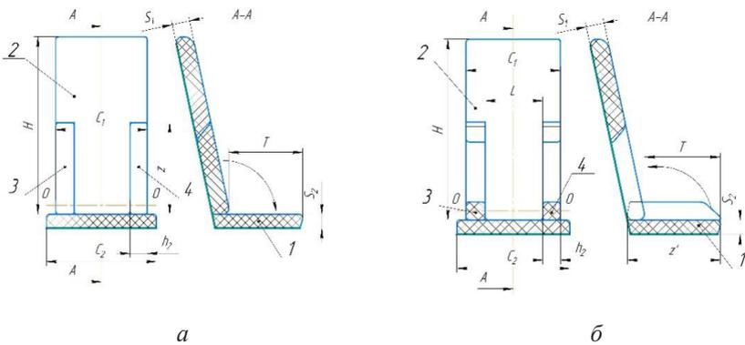
**Figure 3.** Method 1 of chair adaptation in the initial state (a) and after transformation (b).
