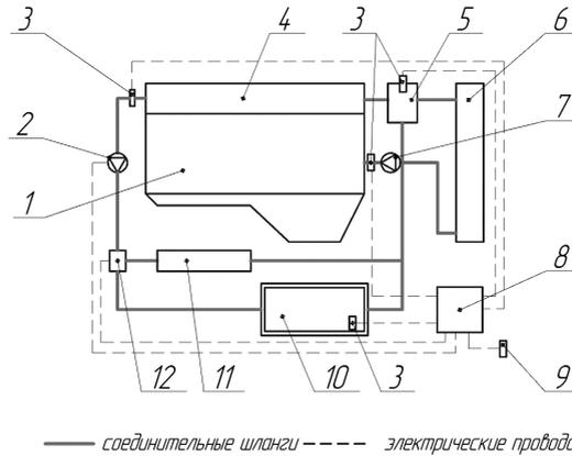
**Figure 1.** A key diagram of the pre-start heating system for a diesel engine: 1 - engine, 2 - an electric pump of the cooling system; 3 - temperature sensors, 4 - head of the cylinder block; 5 - thermostat, 6 - engine cooler; 7 - standard circulating pump, 8 - electronic control; 9 - ambient temperature sensor; 10 - phase transition heat accumulator, 11 - interior heating radiator; 12 - control valve.
