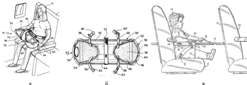
**Figure 2.** Methods for transporting children in the aircraft cabin: in a device for babies [10] (a); device [10] (b); in a child restraint device [11] (b).
