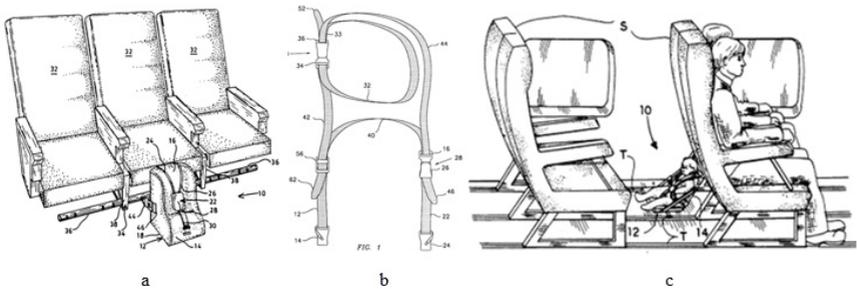
**Figure 1.** Methods for transporting children in the aircraft cabin: in a child seat [6] (a); with fastening with a composite waist belt to an adult [7] (b); in a child seat with fastening to the rails of the seat block [8] (c).
