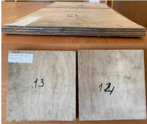
**Figure 6.** Formation of fungal infections (mold) on samples of engineering board No. 13 and No. 14
