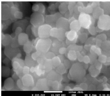
**Figure 2.** *Copper nanoparticles obtained by electric explosion in air.*
