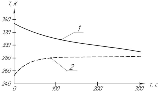
**Figure 4.** Temperature dependence of the heat accumulating substance and the engine on heating timing during the heat accumulator discharge: 1- temperature of the heat accumulating substance; 2 – the engine temperature.
