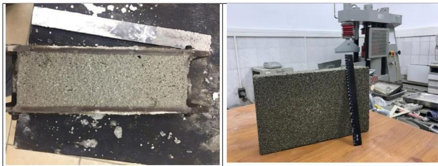
*Figure 2. Perlite cement samples*
