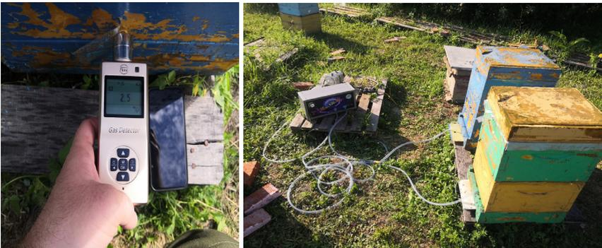
**Figure 1.** Photos of measuring ozone concentration in one of the holes made in the lower part of the hive (left) and the ozonation process itself (right).
