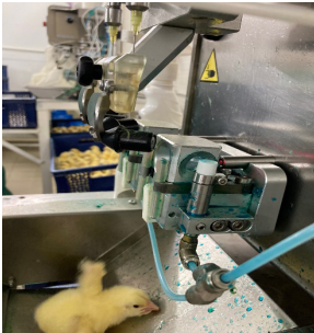
Figure 5. Unclamping the clamping device and moving the chicks down the tray into the prepared crate.
