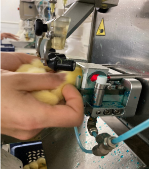
Figure 2. Fixing chicks in prepared grooves of the apparatus with the head of the chicks forward.
