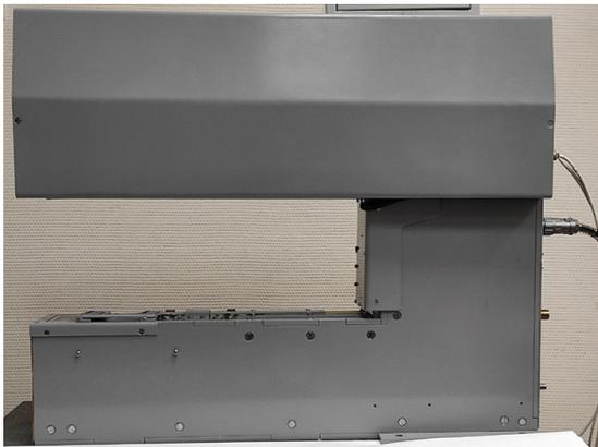
**Figure 2.** Laser thickness gauge TL-3. Dimensions  $W \times H \times L$ , 185 x 596 x 760, mm, weight 75 kg.
