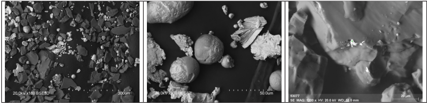
Figure 2. The shape and size of particles of magnetic and non-magnetic iron fractions, and individual quartz grains with metal particles stuck to them after electric pulse crushing
