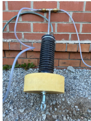
Figure 5. Photo of a bellows generator of pneumatic energy to produce cold and high pressure hydraulic energy to power reverse osmosis desalination plants.
