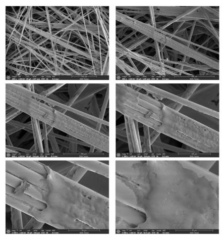
Figures 1 – 6. Micrographs of a material based on basalt fiber at various magnifications.
