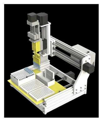
Figure 1. Schematic representation of the developed device for automatic dosing into ELISA plates based on a standard multichannel pipette.
