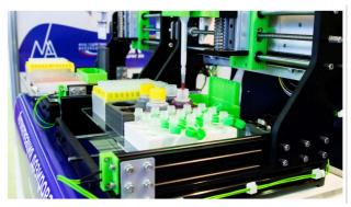
Figure 2. Practical implementation of automatic dosing and mixing of various substances in microvolumes with automatic nozzle change based on a single-channel variable volume pipette.
