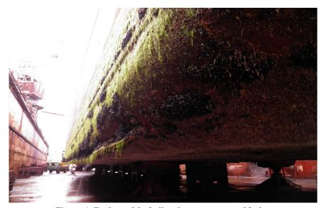
Figure 4. Fouling of the hull with various types of foulers
