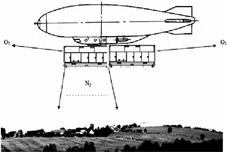
*Figure 1. The use of an agro fire airship to extinguish a forest fire*
