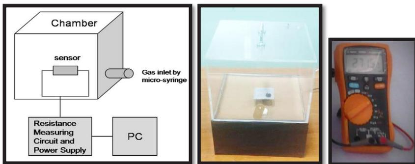
*Figure 3. Explosive testing system chamber and multi-meter*
