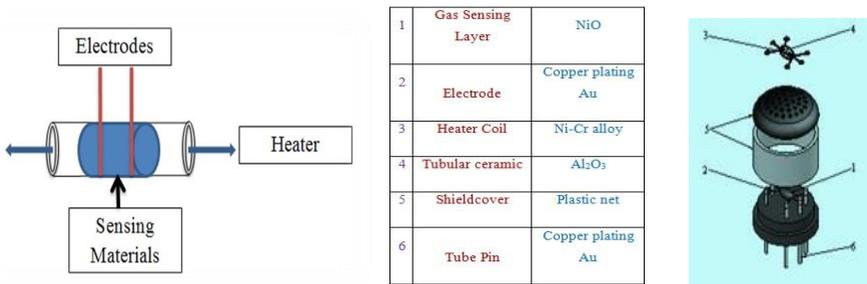
Figure.2 Constructed Tubular ceramic Al<sub>2</sub>O<sub>3</sub> substrate
