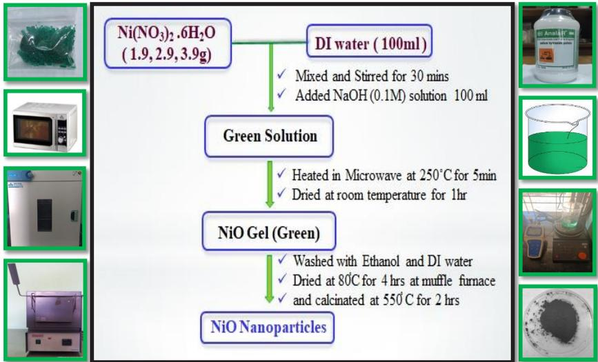
Figure 1. Preparation of Nickel Oxide (NiO) Nanoparticles
