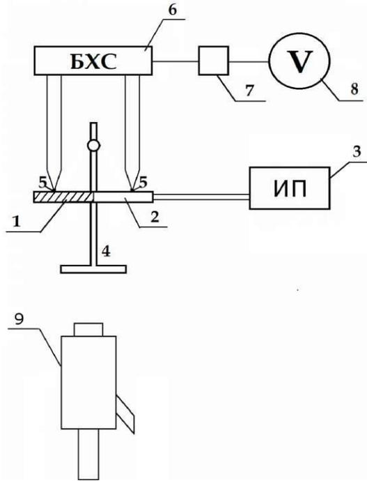
**Figure 1.** Experimental stand for determining the degree of emissivity of zirconium tubes (1 - surface with a known degree of emissivity; 2 - surface under study; 3 - power supply; 4 - tripod; 5 - thermocouples; 6 - cold junction block; 7 - switch; 8 - millivoltmeter; 9 - thermal imager)
