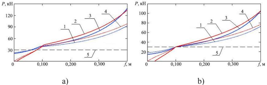
**Figure 2.** Static (1, 4) and dynamic (2, 3) suspension characteristics with a two-chamber single-piston PHS at operating (a) and charging (b) temperatures: 1 - 5 - see fig. 1
