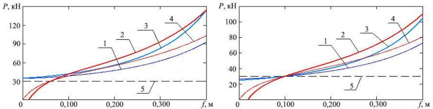
**Figure 1.** Static (1, 4) and dynamic (2, 3) suspension characteristics with a single-chamber single-piston PHS at operating (a) and charging (b) temperatures
