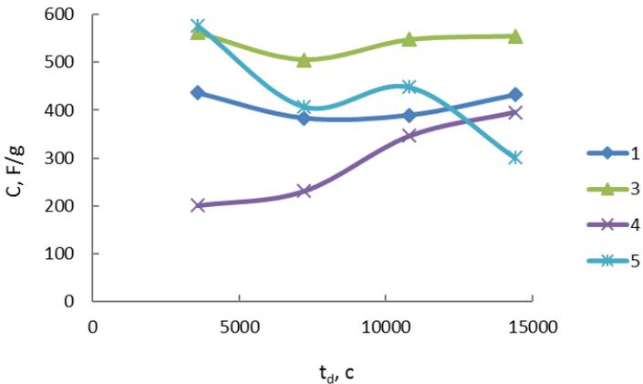
**Figure 4.** Dependence of the specific direct current capacity on the charge time at a current density of 2 mA/cm<sup>2</sup>
