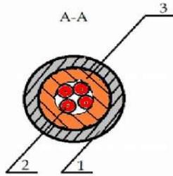
**Figure 3.** Heating element sample (1 - test sample; 2 - nichrome heater in a ceramic tube; 3 - copper tube)
