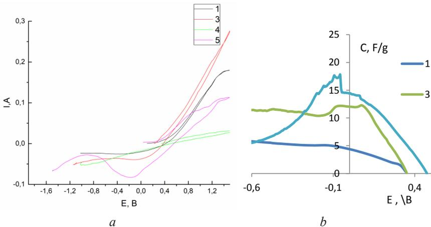
**Figure 1** Cyclic voltammetric dependences of electrodes (a) and dependences of specific voltammetric capacitance on potential (b)
