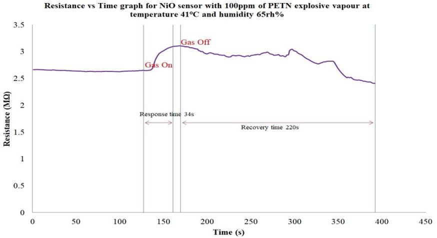
**Figure 4.** Switch behavior of NiO nanoparticles sensor with 100ppm of PETN explosive
