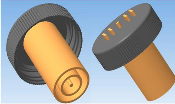
Figure 3. 3D model of the prototype sensor-cover.
