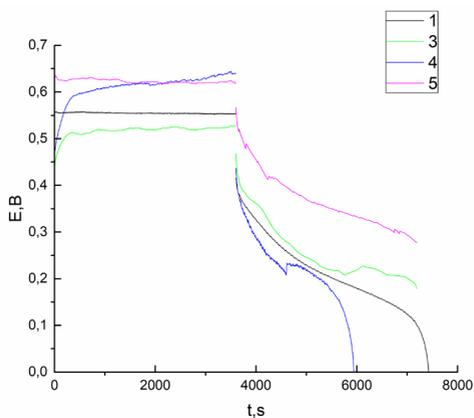
**Figure 2** Charge-discharge characteristics of electrodes at a charge time of 3600 s and a current density of 2 mA/cm<sup>2</sup>
