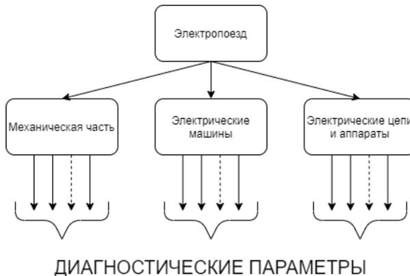
**Figure 1.** Structural diagram of an electric train as an object of diagnosis
