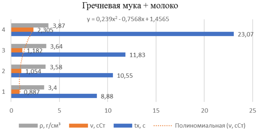
Figure 5. Dependence of the viscosity of the water-milk solution on the density of buckwheat flour
