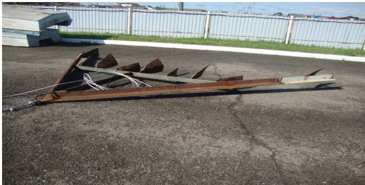
Figure 1. Sludge ripper designed by Sladkovo fish farm. The length of the sharpened edge of the unit is 3 m.
