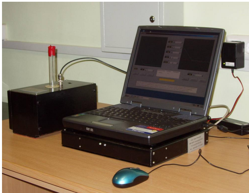
Figure 1. Portable relaxometer NMR NP-2
