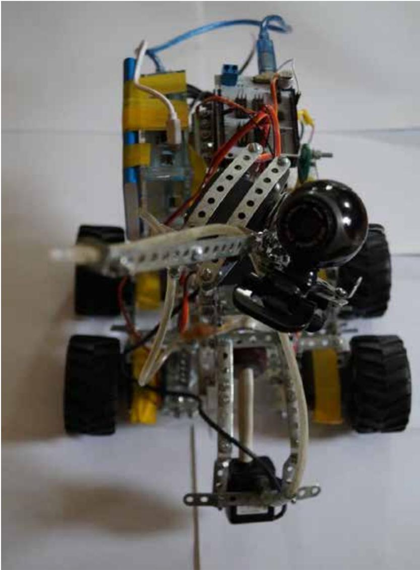
**Fig. 1 – Robot water cannon prototype**
