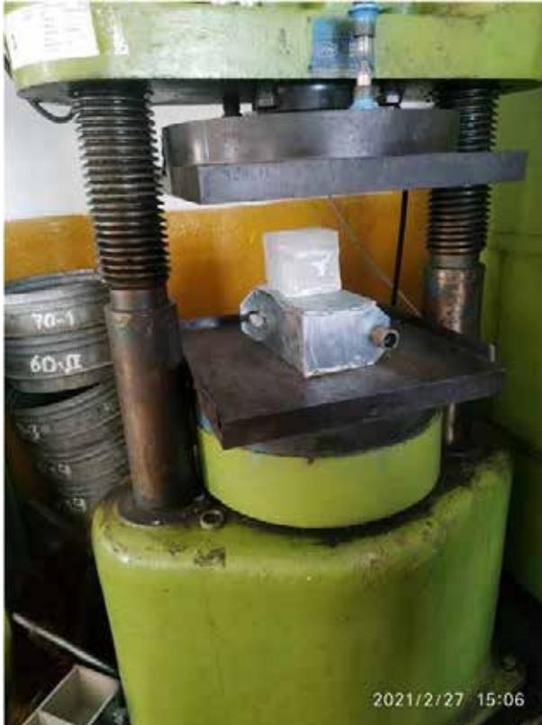
**Fig. 5. Test of ice cubes for strength**
