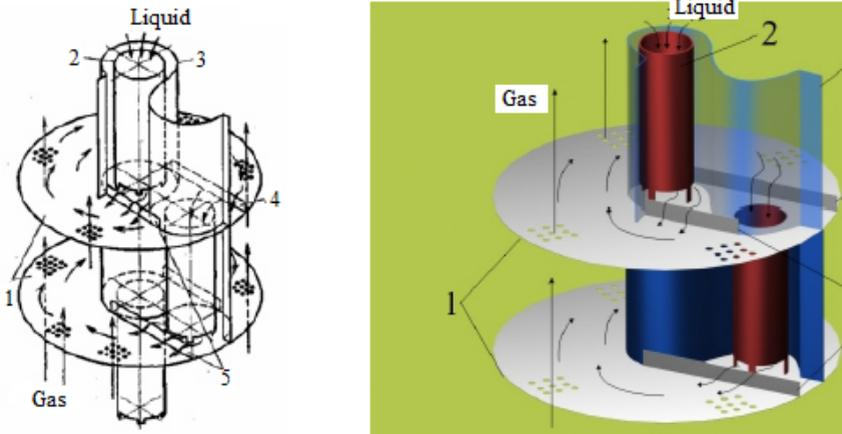
**Figure 4 Perforated plate with an S-shaped baffle**
