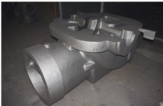
**Figure 1. Casing of the main oil pump MOP**
