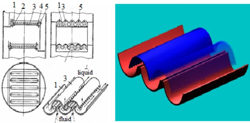
1 – gutter; 2 – supporting rails; 3 – caps; 4 – pins; 5 – drainage
