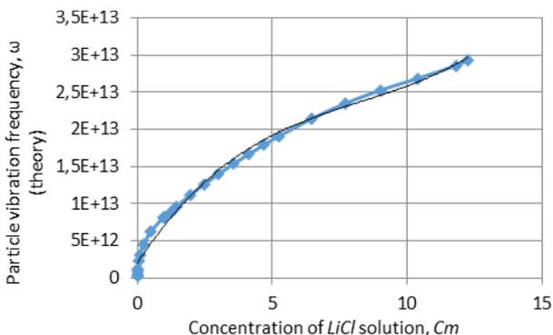
**Fig. 1. Dependence of the theoretical vibration frequencies of lithium chloride particles on the concentration of an aqueous solution of LiCl**
