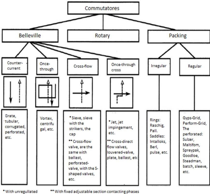
**Figure 1 Classification of contact devices**
