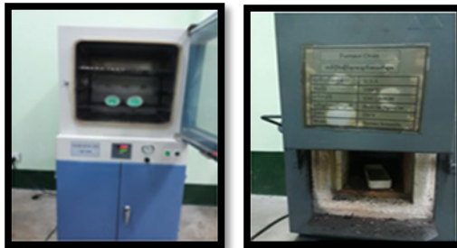
Fig.5. Drying and Calcination Magnesium Hydroxide Precipitate
