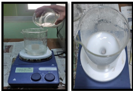
Fig.3. Precipitation of Magnesium Hydroxide
