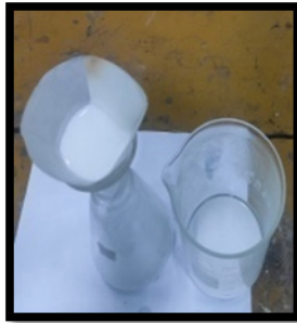
Fig.4. Washing and Filtration of Magnesium Hydroxide Precipitate
