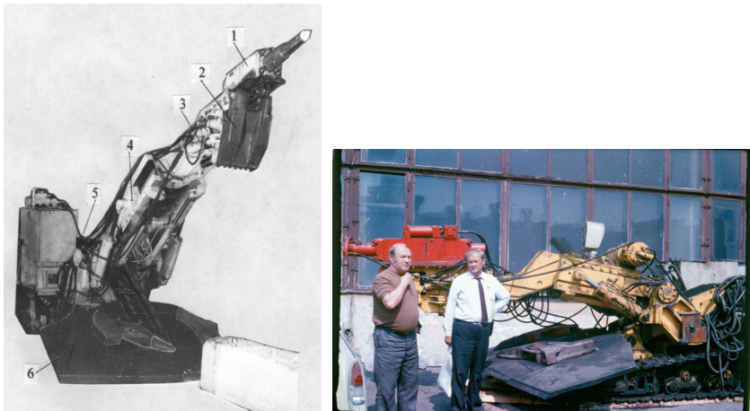
Figure 2. Mining machine "Quartz" with a manipulator and a hydraulic hammer
