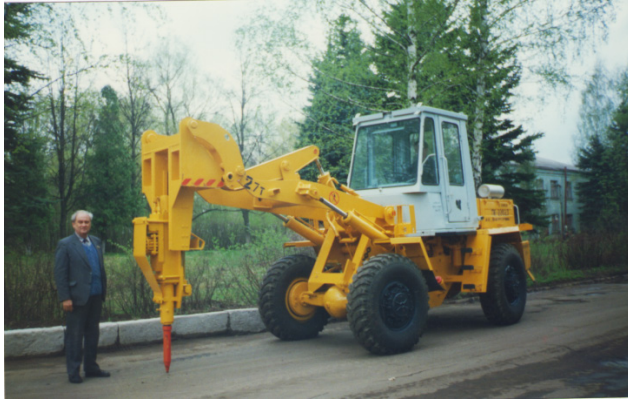
Figure 4. Hydraulic hammer on a wheel loader
